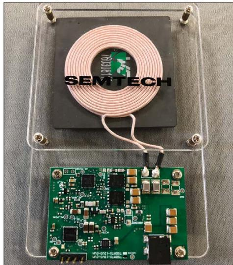
**Airborne Electricity: Coil induces power in battery with Semtech's LinkCharge.**
